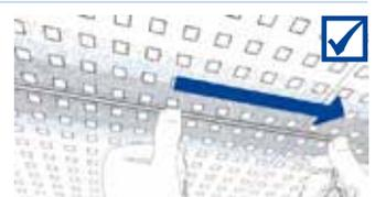
Subsequently coat joint area generously with liquid glue and roll lambskin roller over joint, applying slight pressure.
